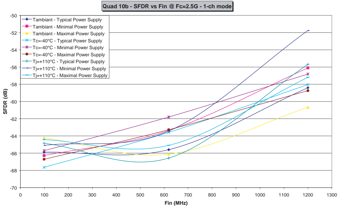
Figure 4-4. SFDR vs Fin in 1 Channel Mode Versus Temp and Power Supply (Min ' all Power Supplies at min value, Max ' all Power Supplies at max Value)
