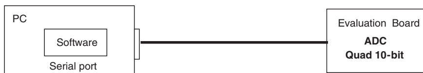
Figure 4-11. QUAD 10-bit 1.25 Gsps User Interface Hardware Implementation
