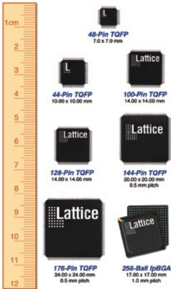
Packages are shown actual size. Dimensions refer to package body size.
