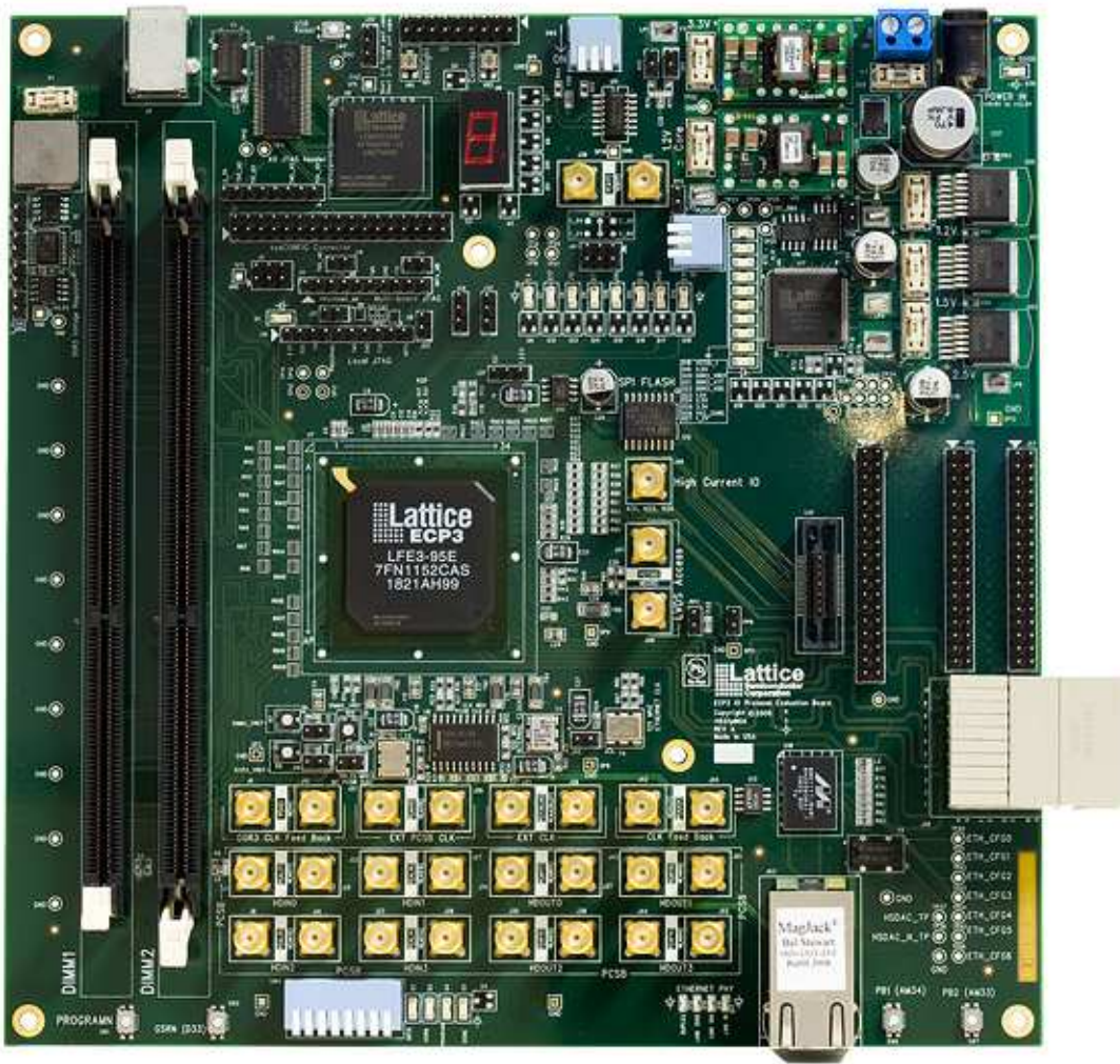
Figure 1: LatticeECP3 IO Protocol Evaluation Board
